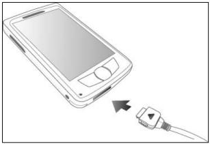
• Insert the charger plug into the jack on the phone.
