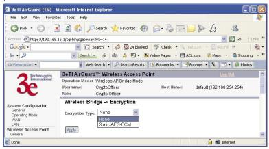
If you select AES-CCM, enter a 128-bit key as 32 hexadecimal digits or use the Key Generator button to automatically generate a randomized key of the appropriate length. This key is initially shown in plain text so you have the opportunity to copy the key. Once the key is applied, the key is no longer displayed in plain text.
