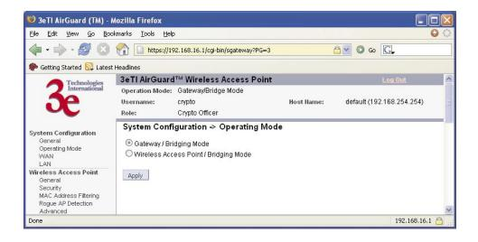
You can then proceed to change the management screens as necessary to reconfigure the device as a gateway. Configuration in gateway mode allows you to set firewall parameters. This is the main difference between the screens you will see in gateway mode and those covered in access point setup as discussed in Chapter 3.
